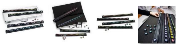
**X-Rite (Macbeth) Farnsworth-Munsell 100 Hue Test** is easy-to-administer with a highly effective method for measuring an individual's color vision. The munsell color test consists of four trays containing a total of 85 removable color reference caps (incremental hue variation) spanning the visible spectrum. Color vision aptitude is detected by the ability of the test subject to place the color caps in order of hue.
